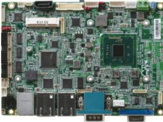
Figure 3 - The GENE-BT05 offers a coastline of connectors that makes migration from legacy solutions simple and cost-effective.
