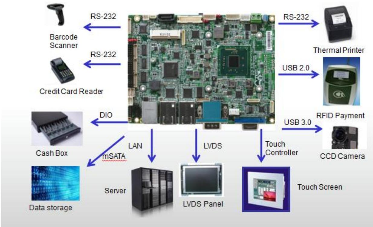
Figure 4 - The rich I/O and expansion features of the GENE-BT05 enable extended functionality for advanced connected POS terminals.
